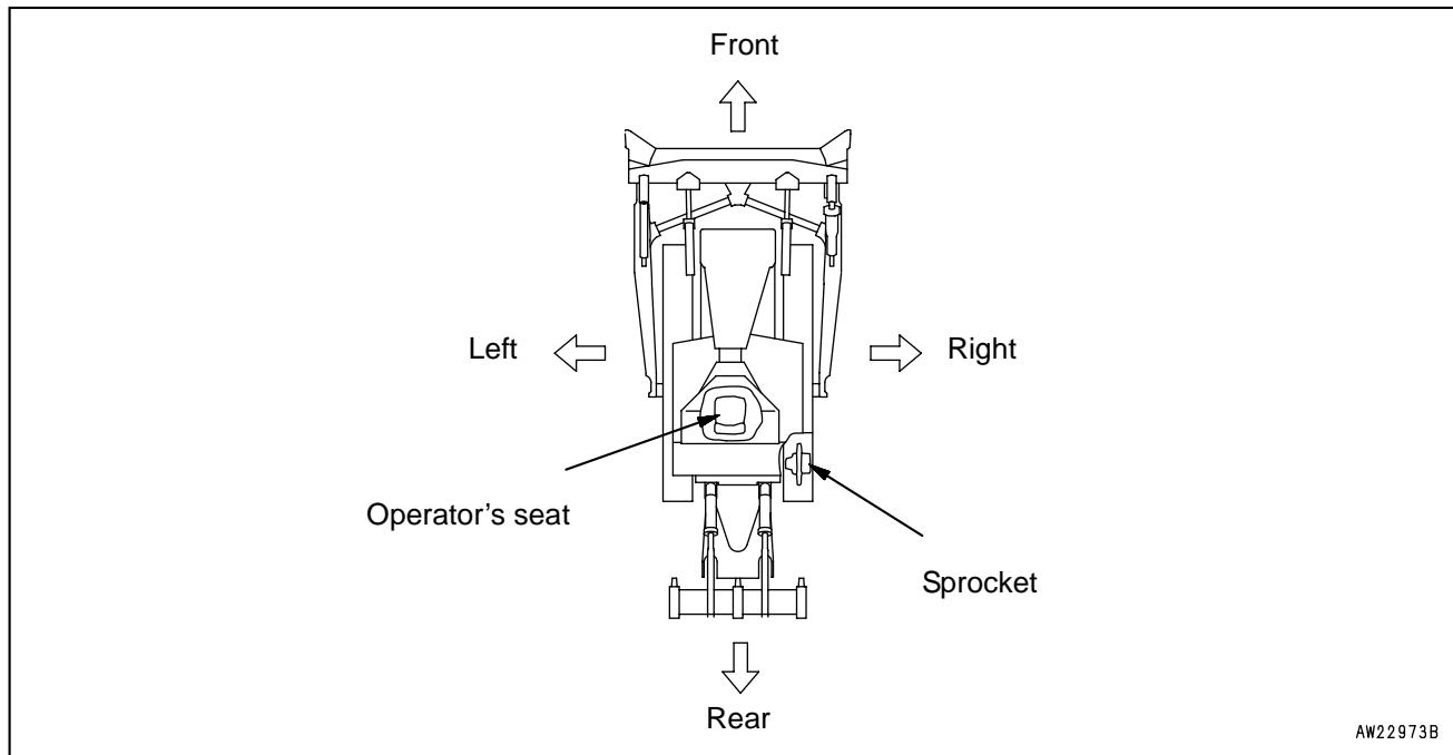
In this manual, the terms front, rear, left, and right refer to the travel direction as seen from the operator's cab when the operator's cab is facing the front and the sprocket is at the rear of the machine.
