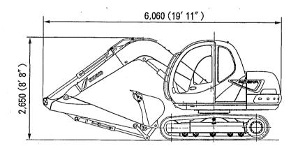
$\odot$ With 3.7m (12' 2") Boom + 1.73m (5' 8") Arm + 0.5m (1' 8") Extension Arm
