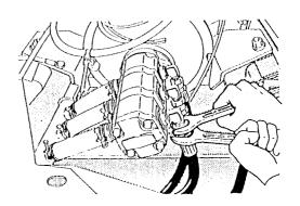
(4) After installing a hydraulic hose or pipe for piping, make sure there is no fluid leakage even when the maximum use pressure is applied 5 or 6 times.
