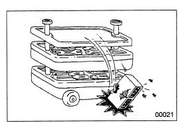
Take care when handling sensors, relays, etc. which are vulnerable to shock and heat. Do not attempt to remove the cover from, or apply paint to, the electronic control unit.
