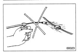
When washing the vehicle, cover the electric system parts and instruments with waterproof material beforehand (Cover with vinyl sheet or the like). Keep water away from harness wire connectors and sensors. If any of them should get wet, wipe them off immediately.
