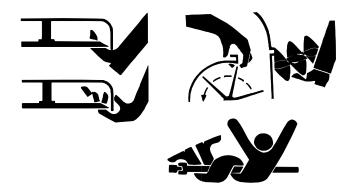
Keep hands and feet away while machine is running. Shut off power to service, lubricate or remove mower blades, augers or PTO shafts.
