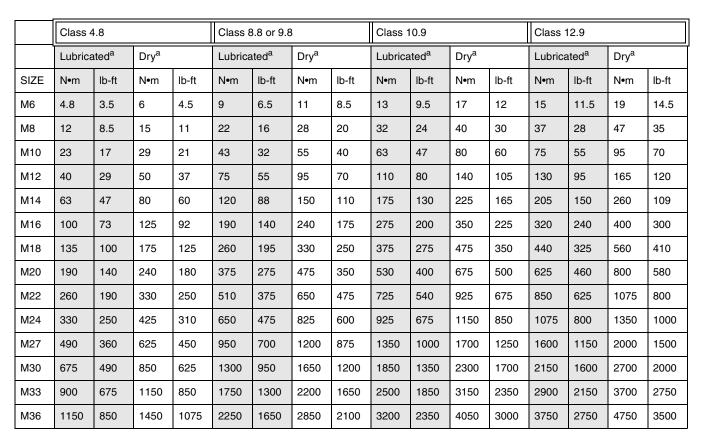
DO NOT use these hand torque values if a different torque value or tightening procedure is given for a specific application. Torque values listed are for general use only and include a  $\pm$  10% variance factor. Check tightness of fasteners periodically. DO NOT use air powered wrenches.
