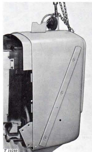
Fig. 20-5-2—Removing Grille Housing
