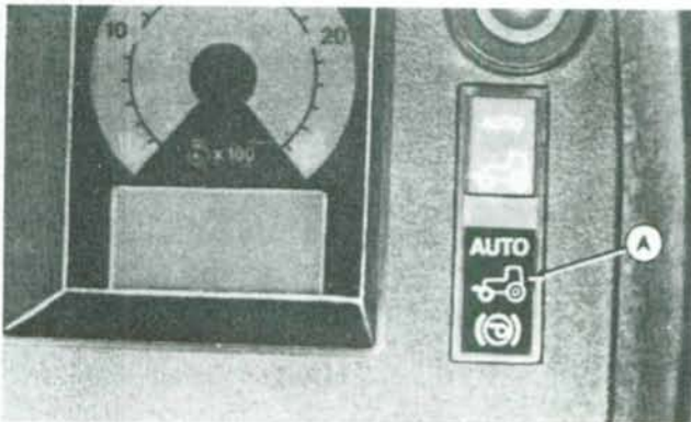
Fig. 6—The three-position rocker switch (A) for front-wheel drive is located on right side of instrument panel.
