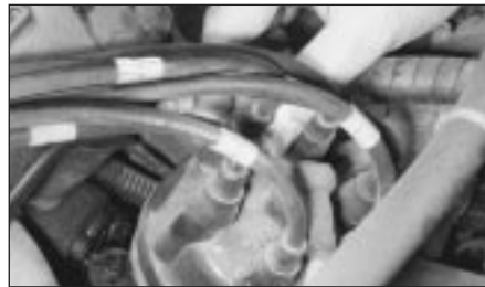
B Check that the spark plug HT leads are securely connected by pushing them onto the plugs and distributor connections.
