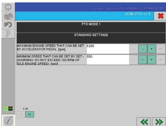
**MAXIMUM ENGINE SPEED THAT CAN BE SET BY ACCELERATOR PEDAL (RPM):** The maximum engine speed obtainable in PTO mode can be set with the accelerator pedal.
