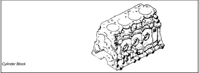
The cylinder block is a complex structure with cooling water and lubricating oil passages, and crankshaft supports in the lower part. The cylinder block is made of cast iron because it has to be strong enough to resist not only high temperatures, but also the high pressure gasses generated in the cylinders. It also needs to have sufficient corrosion resistance to withstand these gasses.
