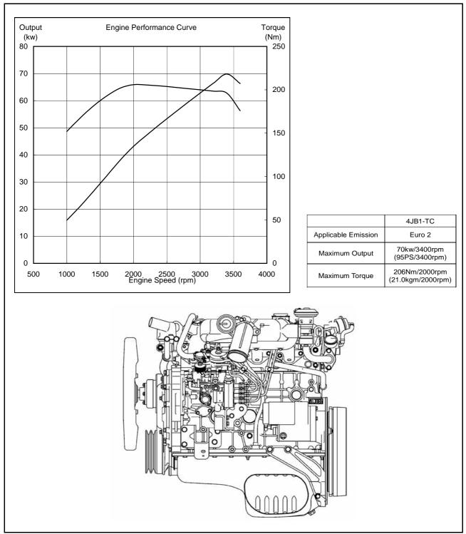
The four cycle direct injection 4JB1-TC engine features two valves per cylinder that are operated via a single camshaft fitted to the engine block.
