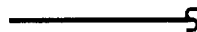
Wavy line means the wire is broken by the binding of the book but continues on the next page
