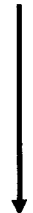
Arrow means wire connects to another circuit; shows direction of current flow
