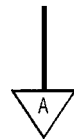
Circuit is continued where indicated; arrow shows direction of current flow and is repeated where circuit continues
