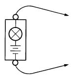
A self-powered test light is only used on an un-powered circuit. First disconnect the battery or remove the fuse that feeds the circuit you are working on. Select two points along the circuit through which there should have continuity. Connect one lead of the self-powered test light to each point. If there is continuity, the test light's circuit will be completed and the bulb will go on.
