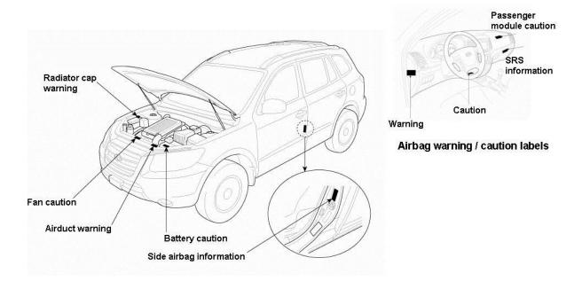
During pre delivery inspection and service the condition of the warning labels should be checked. Various warning labels such as SRS-warning, Air duct warning, Fan and battery caution are available. Please refer to the shop manual for more details about their location.
