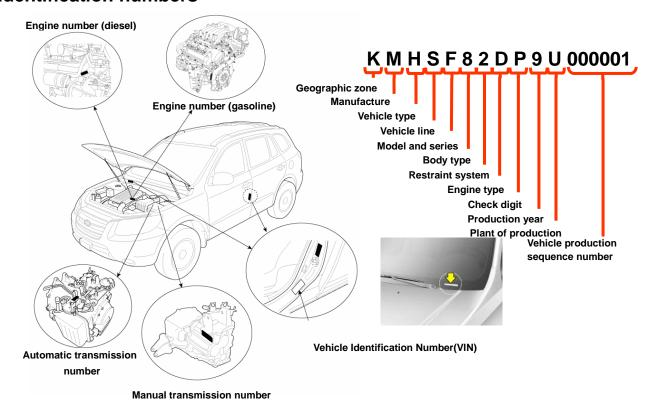
Identification marks are stamped on to various vehicle components such as the engine, transmission and vehicle body. The Vehicle Identification Number (VIN) reveals the following information (sample CM):
