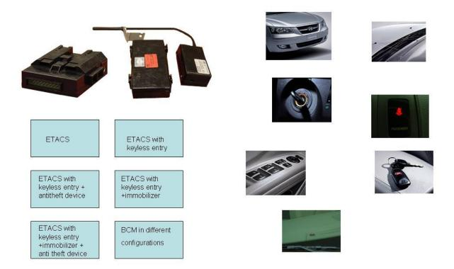
The electronic time and alarm control system (ETACS) is a special control system for time and alarm related functions such as:
