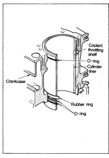
water jacket holes to around all cylinders. After cooling the cylinders, the coolant reaches the cylinder head
