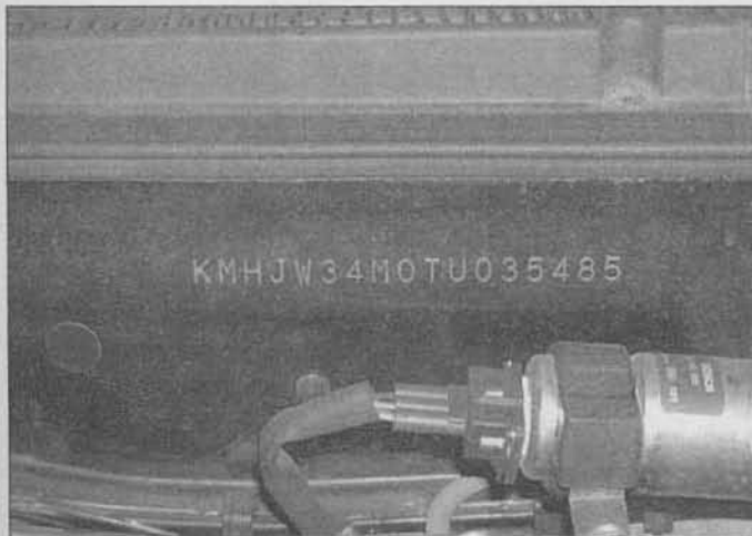
The Vehicle Identification Number (VIN) is also stamped into firewall in the engine compartment
