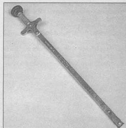
Hydraulic lifter removal tool
