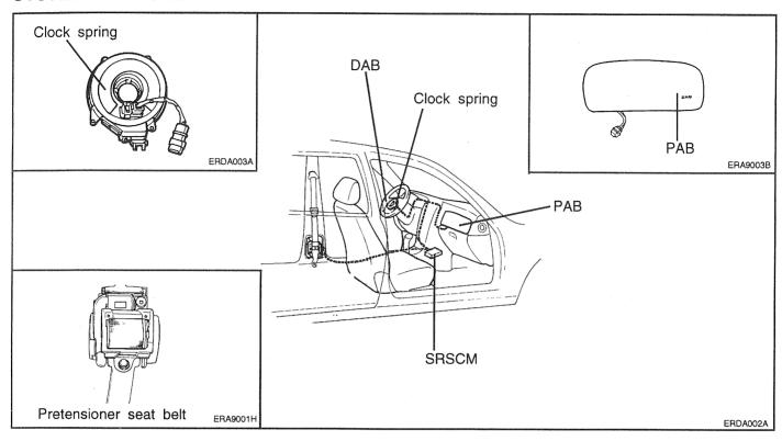
The Hyundai ACCENT(VERNA/EXCEL) is equipped with a Supplemental Restraint System (AIRBAG) to provide the vehicle's driver and/or the front passenger with additional protection than that offered by the seat-belt system alone, in case of a frontal or lateral impact of sufficient severity.
