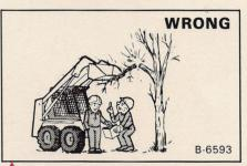
Never work on loader with lift arms up unless lift arms are held by a lift arm support device.
