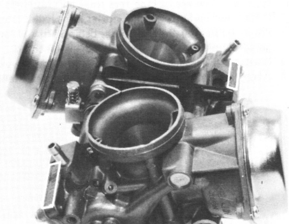
The carburetor identification number is on the carburetor body intake side.
