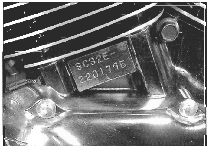
The engine serial number is stamped into the right side of the crankcase, below the rear cylinder
