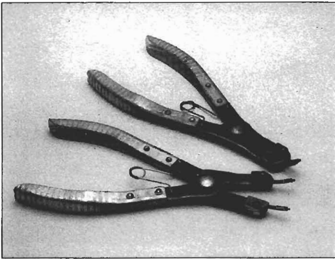
Snap-ring pliers (top - external; bottom - internal)
