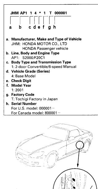
Vehicle Identification Number and Federal Motor Vehicle Safety Standard Certification. Vehicle Identification Number and Canadian Motor Vehicle Safety Standard Certification.
