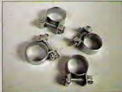
Notice how these fuel-injection hose clamps don't have the ridges in them that you would normally find in a standard hose clamp.
