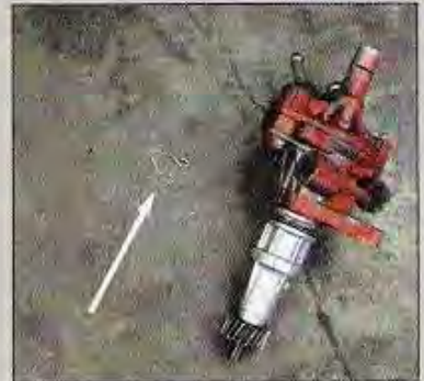
The clip pictured to the left will slip into the groove on the top of the vehicle speed sensor shown on the right. Without it, the cable will slip out of place.
