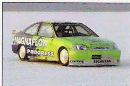
The world's fastest Honda is the Progress Suspension Landspeed Civic. It relies on huge horsepower from a highly modified B-series engine. At over 200 mph, the stock D-series Civic engine just couldn't cut it. (Photo Courtesy of Progress Suspension)
