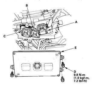
11. Disconnect the PCM connectors A, B, and C.
