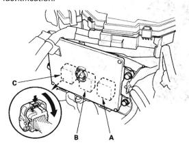
6. When diagnosis/troubleshooting is done at the PCM connector, use the terminal test port (A) above the terminal you need to check.
