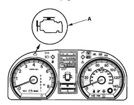
2. If the MIL stays on, connect the HDS to the data link connector (DLC) (A) located under the driver's side of the dashboard.
