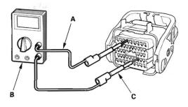
8. Gently contact the pin probe (male) at the terminal test port from the terminal side. Do not force the tips into the terminals.
