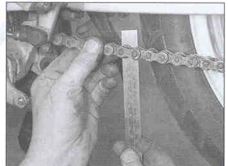
1.3 Push up on the chain and measure the slack
