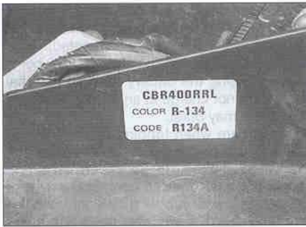
The colour code label is under the passenger seat
