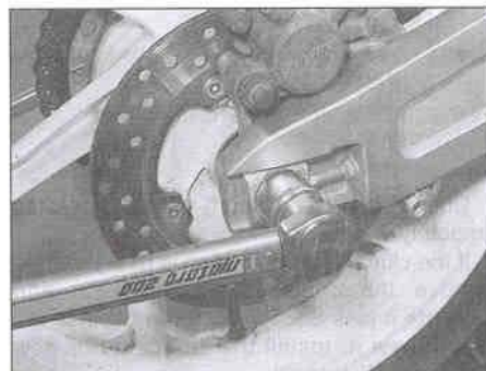
1.12 Tighten the axle nut to the specified torque
