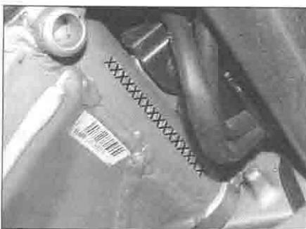
The frame number is stamped into the right-hand side of the steering head
