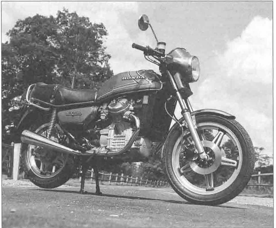
The CX500 – Honda's first V-Twin and a favorite choice of dispatch riders
