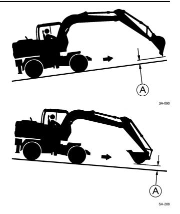
Driving across the face of a slope or steering on a slope may cause the machine to skid or overturn. If the direction must be changed, move the machine to level ground, then, change the direction to ensure sage operation.
