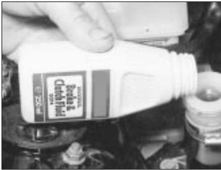
4.15 Adding hydraulic fluid to the clutch fluid reservoir
