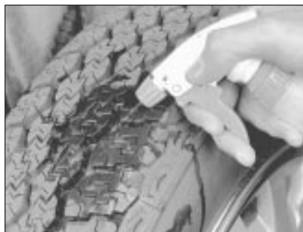
5.4b If the valve core is tight, raise the vehicle, and spray a soapy water solution onto the tread as the tyre is turned slowly - leaks will cause small bubbles to appear
