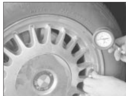
5.8 To extend the life of the tyres, check the air pressure at least once a week with an accurate gauge (don't forget the spare!)
