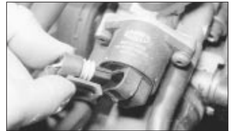
C Check the idle speed stepper motor wiring plug for security.
