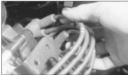
A Check that the spark plug HT leads (where applicable) are securely connected by pushing them home.
