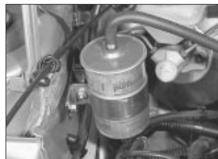
32.2 Fuel filter fuel hose and retaining clamp locations
