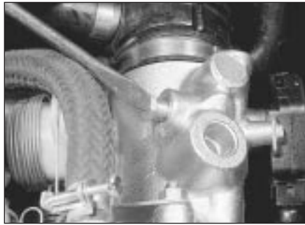
28.22a Idle speed air screw adjustment on the LE2-Jetronic fuel injection system
