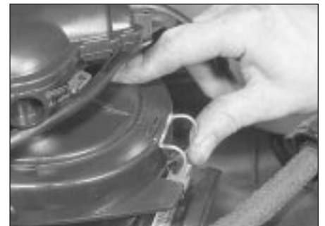
26.5b . . . or release the spring clips . . .
