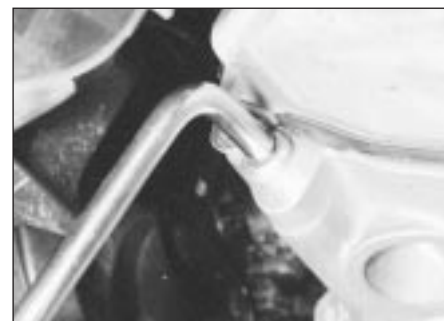
21.3 Using a square section wrench to unscrew the transmission filler/level plug (MA transmission shown)
