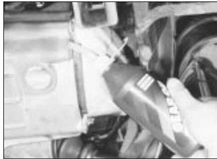
21.4 Topping-up the transmission oil level
