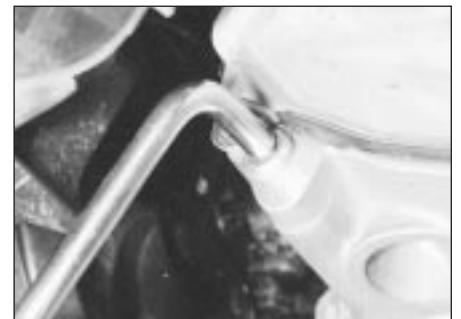
21.3 Using a square section wrench to unscrew the transmission filler/level plug (MA transmission shown)
