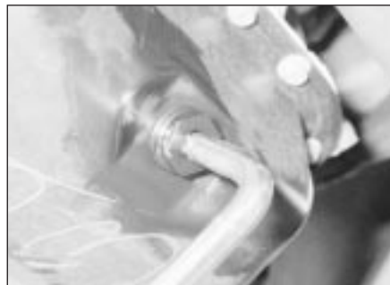
3.3 Slackening the sump drain plug with a square section wrench
