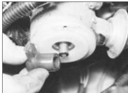
27.9 Remove the rotor arm from the distributor for inspection
