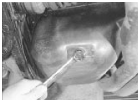
6.4 Removing the sump drain plug
