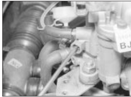
11.4c Adjusting the idle speed - Varajet carburettor
