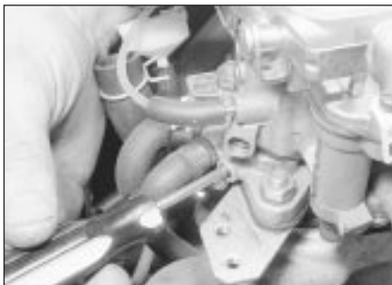
11.7c Adjusting the mixture (CO) setting - Varajet carburettor
