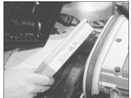
24.13 Fitting a new air cleaner element - 2.0 litre 16-valve models
