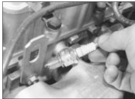
7.5 Removing a spark plug - 1.6 litre engine shown
