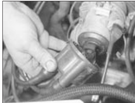
10.9a Remove the distributor cap . . .
