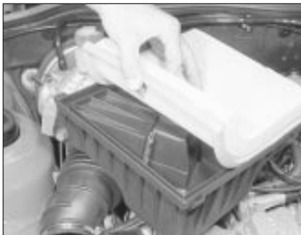
24.9 On fitting, ensure the element is correctly seated in the cover groove
