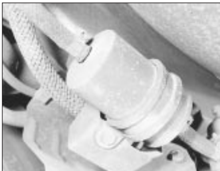
25.3 Fuel filter showing mounting and hose connections
