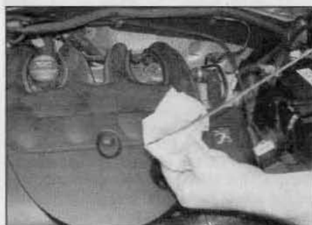
2 Using a clean rag or paper towel, wipe all the oil from the dipstick. Insert the clean dipstick into the tube as far as it will go, then withdraw it again.
