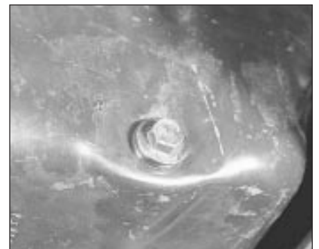
8.2 Sump drain plug location
