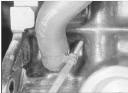
35.1 Loosening the crankcase ventilation hose clip - CVH models
