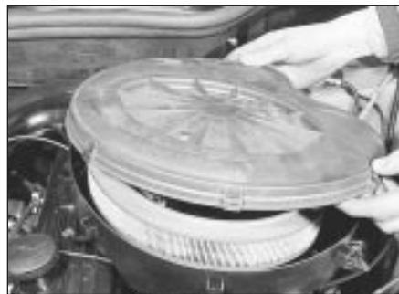
38.2 . . . release the spring clips, and lift off the cover for access to the element
