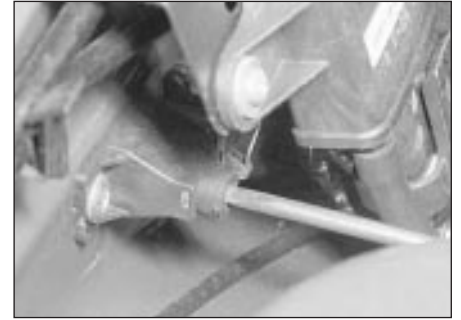
16.34b . . . to enable mixture adjustment - DOHC models
