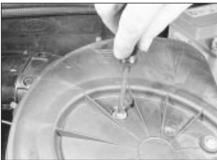
38.1 Remove the air cleaner cover screws . . .
