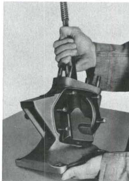
Fig. FO502—To remove the steering worm shaft from main housing, remove lower stud and withdraw shaft through side opening as shown.
