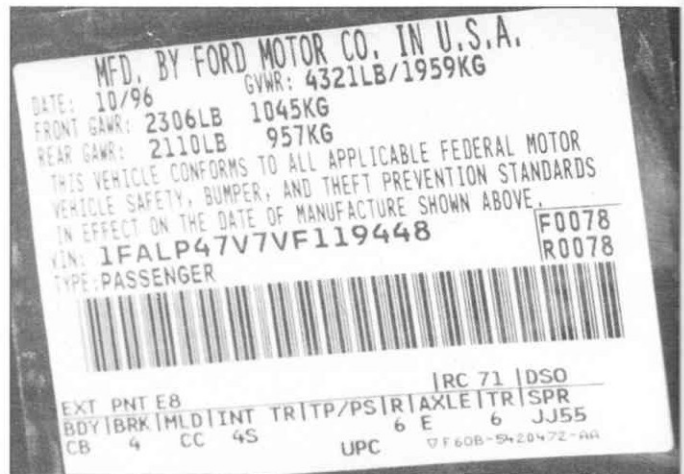
The vehicle certification label is affixed the to the driver's side door pillar
