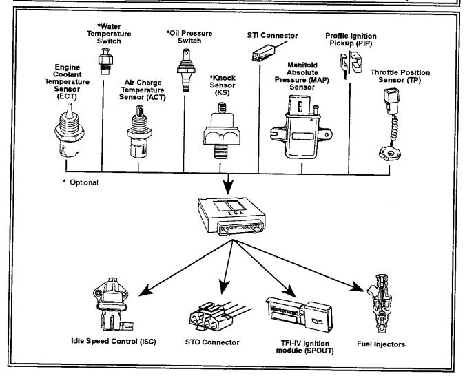
FORD's EEC-IV system is an electronic engine control system that consists of a network of electronic and electromechanical components. This system will continuously vary engine operation in order to meet programmed engine operating parameters.
