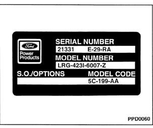
An engine code decal is attached to the engine front cover. The symbol code on the decal identifies each engine for determining parts usage.
