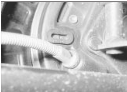
4.4a Remove the inspection plug from the rear brake backplate . . .
