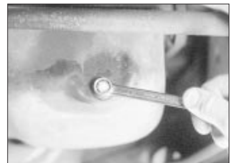
3.3 Removing the sump drain plug
