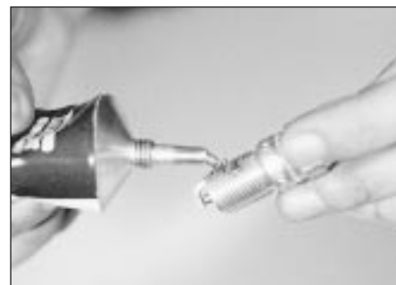
12.5 Lightly grease the spark plug threads before fitting
