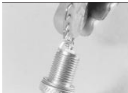
12.2c Adjusting a spark plug electrode gap with a special tool
