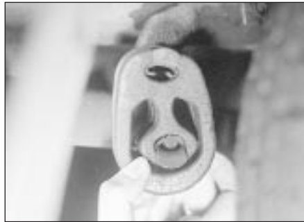
7.1 Inspect the exhaust system rubber mounting
