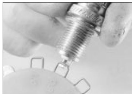
12.2b Measuring a spark plug electrode gap with a wire gauge
