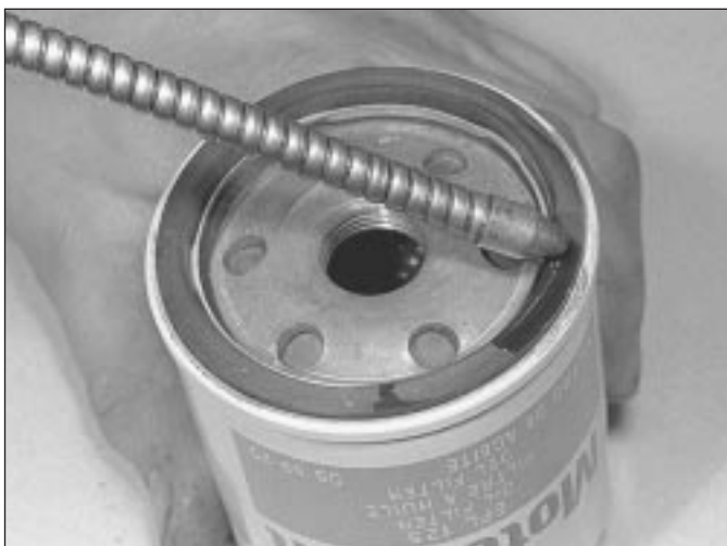
3.10a Lubricate the filter's sealing ring with clean engine oil before installing the filter on the engine
