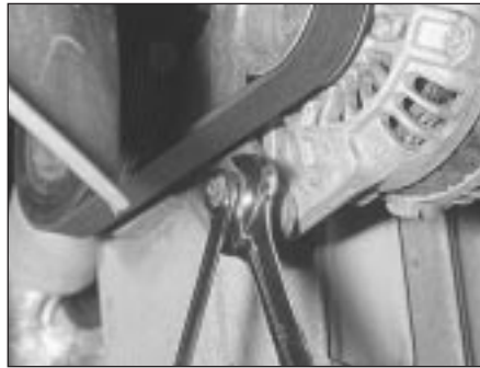
4.12b When the tension is correct, hold the adjuster nut, and tighten the central bolt securely to lock the adjuster arm
