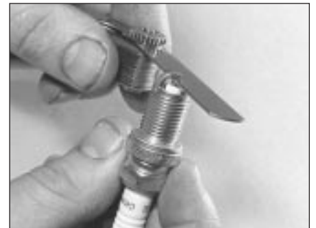
21.12a Measuring a spark plug gap with a feeler gauge
