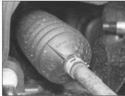
10.2c Check the condition of the steering rack gaiters
