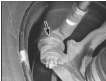
10.2a Check the condition of the track rod end balljoint dust cover (arrowed)
