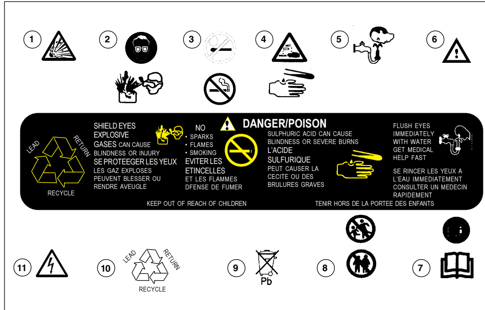
Fig. 1—Typical Battery Labelling
