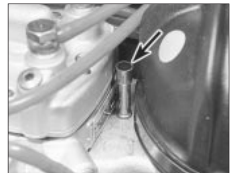
10.21 K-Jetronic system mixture adjustment screw location (arrowed)
