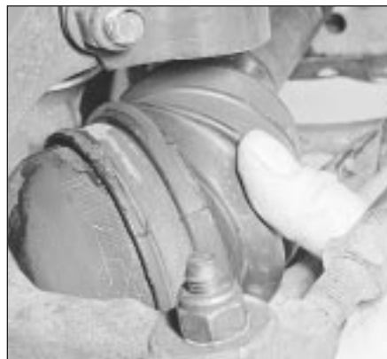
29.3 Checking driveshaft outer joint rubber bellows
