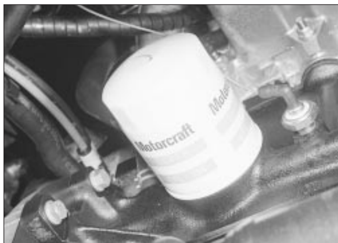
6.7 Oil filter location - CVH engine
