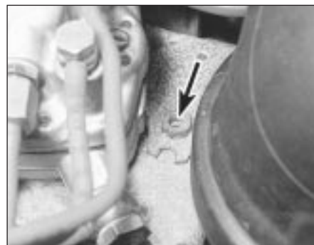
10.33 KE-Jetronic system mixture adjustment tamperproof plug (arrowed)
