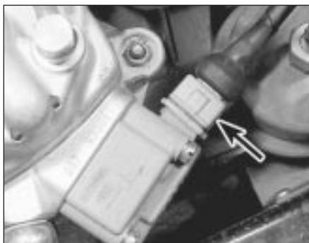
10.29 Pressure actuator wiring multi-plug (arrowed) - KE-Jetronic system
