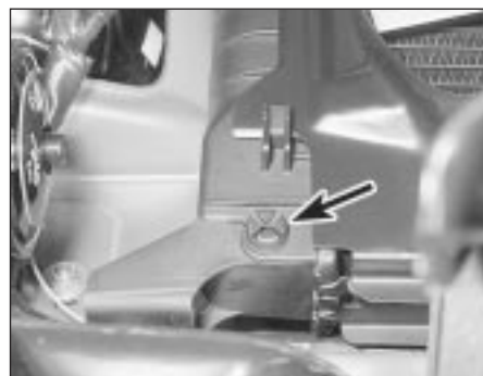
33.3 Radiator drain plug location (arrowed)
