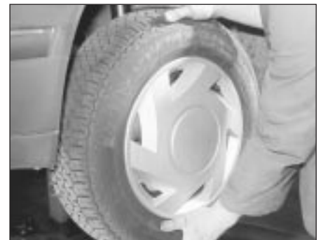
18.3 Rocking the roadwheel to check steering/suspension components
