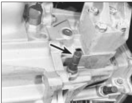
26.6 Selector shaft locking mechanism cap nut (arrowed)
