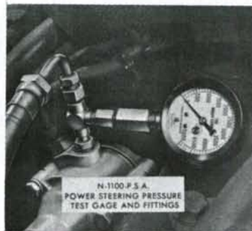
Fig. FO14—Method of installing pressure gage in series with the power steering pump pressure line.
