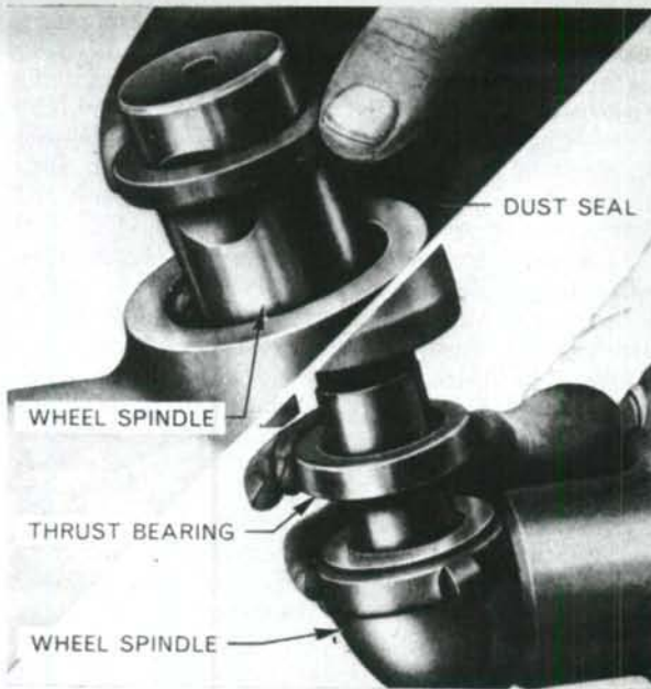
Fig. 2—Top view shows proper installation of dust seal on spindle after spindle is installed in axle extension. Lower view shows proper installation of thrust bearing on spindle prior to installing spindle in axle extension.
