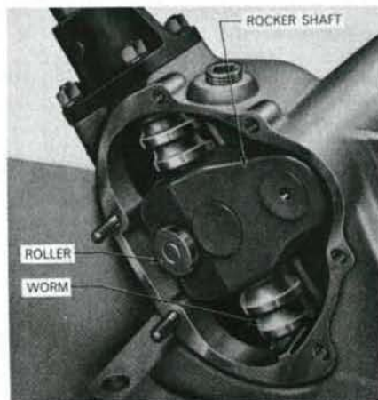
Fig. 4—View of steering gear assembly with side cover removed. Roller moves in slot in side cover.
