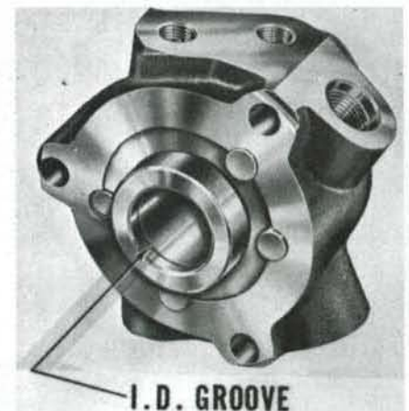
Fig. 15—Insert control valve spool in housing so that identification notch will be towards top end of steering shaft.
