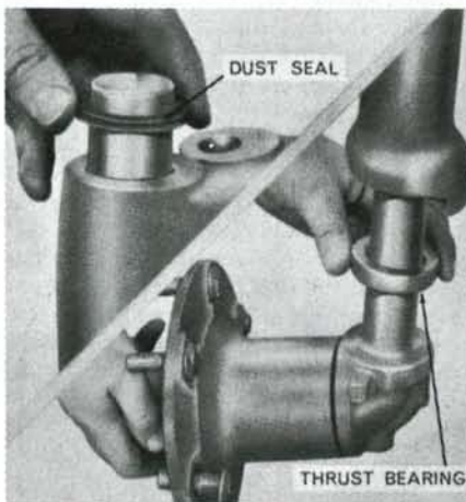
Fig. 2—Top view shows proper installation of the dust seal on upper end of spindle before installing steering arm. Lower view shows installation of thrust bearing on spindle before installing spindle in axle extension.
