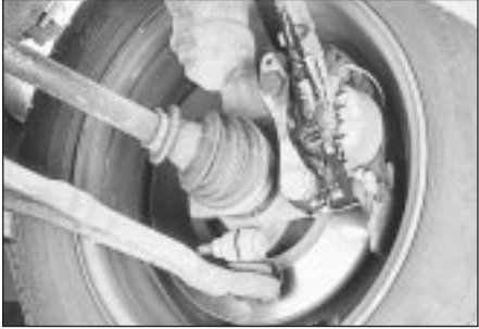
A leak occurring at a wheel is almost certainly brake fluid.
