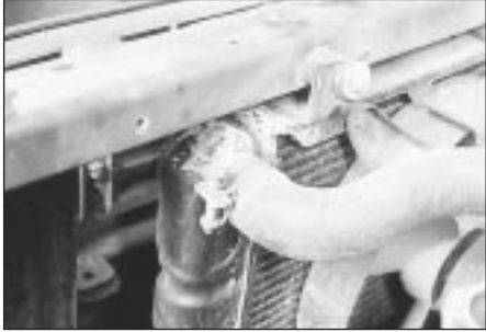
Leaking antifreeze often leaves a crystalline deposit like this.
