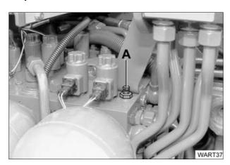
1. Loosen stopcock item A (stopcock is labelled AV2 in further documents and circuit diagrams) on top of central control block by approx. 1 turn anti-clockwise.
