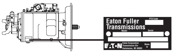
All Eaton® Fuller® Transmissions are identified by the model and serial number. This information is stamped on the transmission identification tag and affixed to the case.
