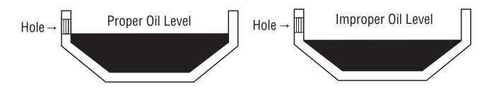
When checking the transmission lubricant there are two important points to know: where to check the lubricant and what the proper lubricant level is. Always be cautious when checking the transmission lubricant as it may be hot.
