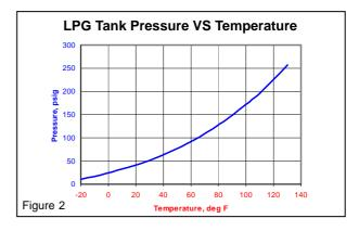
With 128 PSIG vapor pressure acting against the liquid propane the boiling point has been raised to slightly more than 80 deg. F / 27 deg. C.
